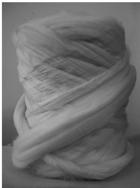
Figure 1 Extrafine merino wool used as substrate for silver deposition.
